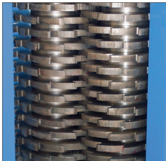
Twin shaft cutting chamber.
