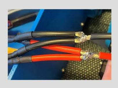
Soldering needed to be done to connect the motors and the VESC
