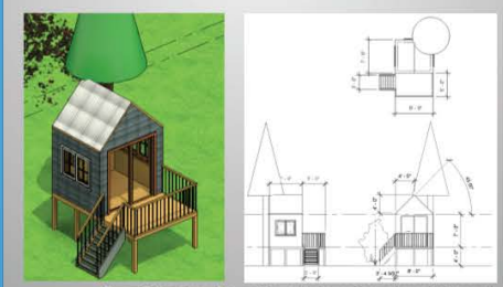
Figure 6: Top, front, side, and isometric views of a tree house Revit model
