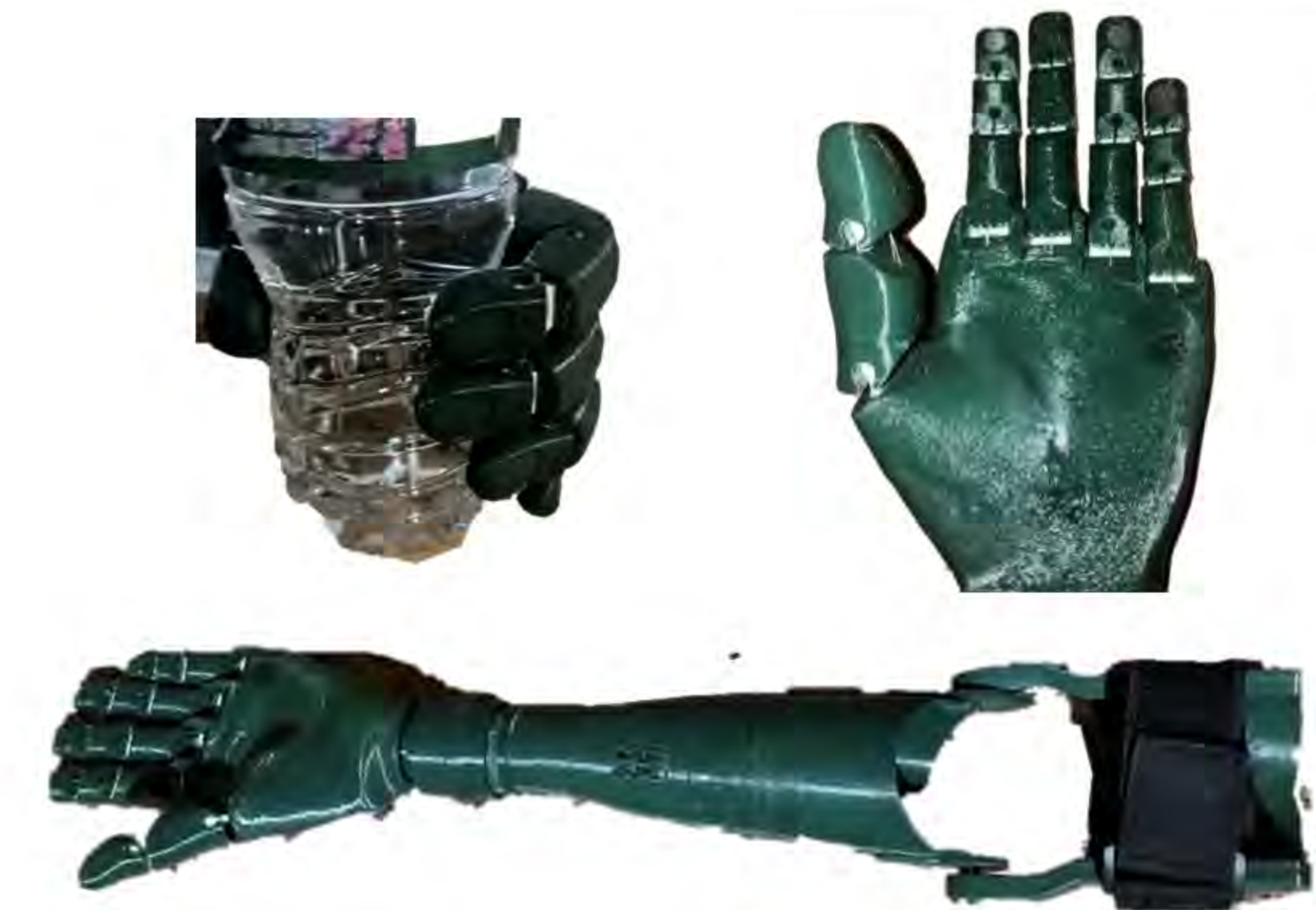
Figure 8: Fully Assembled Updated Body-Powered Prosthesis
